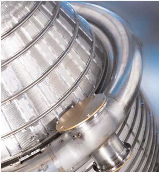
Close-up of the inlet through which Turbine Exhaust Gas (TEG) supersonic film is fed to cool the metal skirt.
