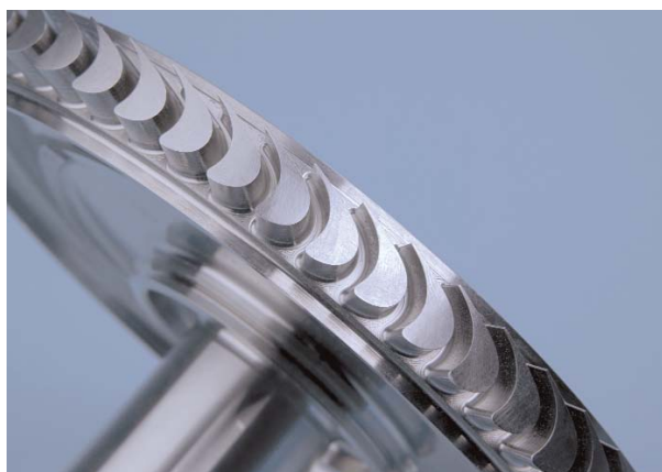
Vinci LOX shaft and blisk Vinci rotors are shroudless blisks (BLade Integrated diSKs) where the blades are made by radial milling. Depicted is the LOX rotor milled in Inconel 718.
