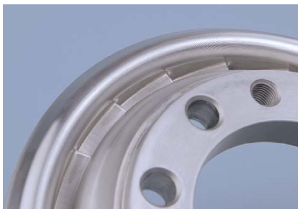
Stator Vinci LH2 The outer shrouds of the Vinci stators are brazed to the inner ring of radially milled vanes, giving a smooth, strong and ductile joint. Both stators are made in stainless steel (Nitronic 40). Patented manufacturing technique.
